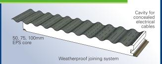
"The Roof" is a durable three-tiered roofing material which bonds a high tensile roof sheet and a smooth underskin/ceiling with an insulating polystyrene core. Roof sheets and beams are made-to-measure and it comes ready-to-erect.
